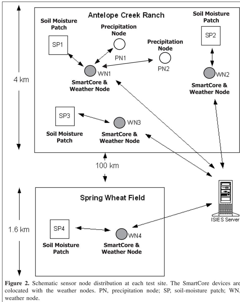
**Figure 2.** Schematic sensor node distribution at each test site. The SmartCore devices are collocated with the weather nodes. PN, precipitation node; SP, soil-moisture patch; WN, weather node.
