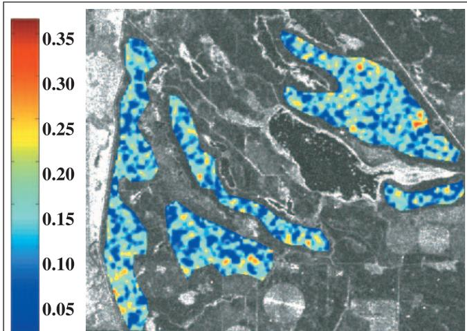
**Figure 4.** Estimated surface soil-moisture map for the Antelope Creek Ranch, Alberta, derived from 100 m ASAR imagery acquired on 18 August 2004. The soil-moisture units are fractions. The image map area is approximately 4 km × 4 km.
